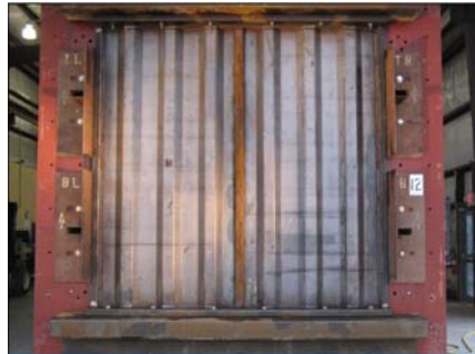
Figure 7 – Wall Panel Of SWCP Construction Used In Physical Test Phase
